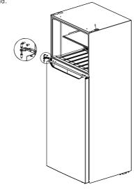
7)Install the door of freezer on the middle hinge, take out the left upper hinge and the cover for the left upper hinge from the accessory bag, install the left hinge and tighten the screws, install the cover for the left upper hinge and tighten the screw, install the right sensor in the original left hole cover, and then fix the hole cover on the right box.
