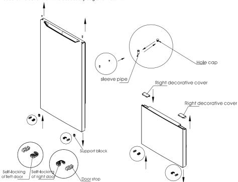
6)Install the door of refrigerator chamber on the lower hinge, the middle hinge on the left side of the refrigerator and tighten the screws, and place the shaft sleeve well. Install the plug pin in the hole on the middle beam at the other end.
